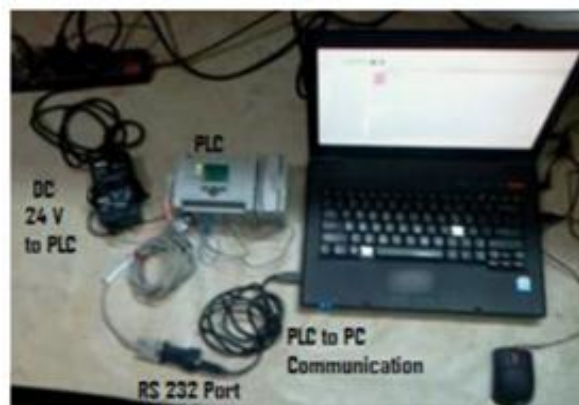
Fig 4: PLC to PC Communication
