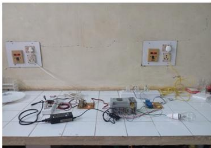
Fig. 7: Testing Of I/O Modules
